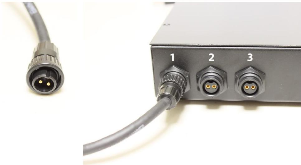
Each cable serves up to ten stand lights and occupies one DMX address or one bank. There are three DMX addresses and three cables per decoder. The left connector, bank 1, corresponds with the primary DMX address (as configured by the DIP switches). The center connector, bank 2, is the primary address plus one. The right connector, bank 3, is the primary address plus two.
